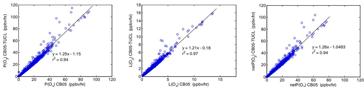
**Figure 1.** Comparison ozone production rate ( $P(O_3)$ ) (left), ozone loss rate ( $L(O_3)$ ) (middle), and net ozone production (net  $P(O_3)$ ) (right) in the old (CB05) and updated (CB05-TUCL) versions of the chemical mechanisms.
